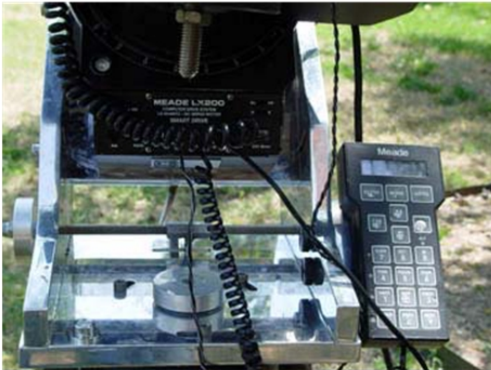
Picture 4: Top view of the wedge and front view of the control panel for the LX200
